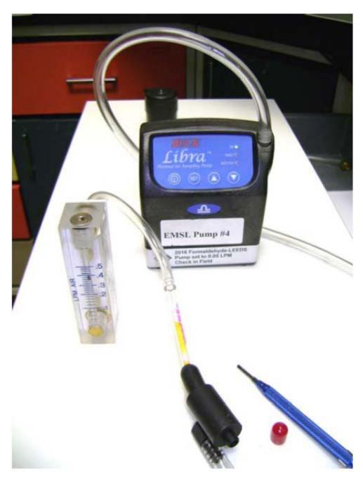
...and read the flowrate. It should be between 0.05 and 0.5 Liters per minute (lpm), the **OPTIMAL** flowrate is **0.3 lpm**. If it is not at 0.3 lpm, carefully use a small screwdriver to adjust the flow using the screw on the low-flow adapter FIRST;
