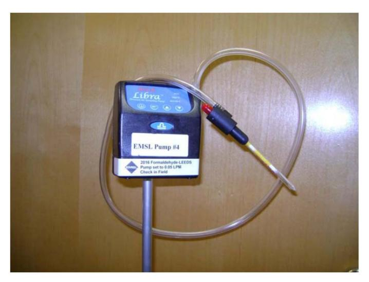
12) Periodically check to ensure that the pump is running. A pump that has failed and was left unattended during the sampling period will need to be discarded;
