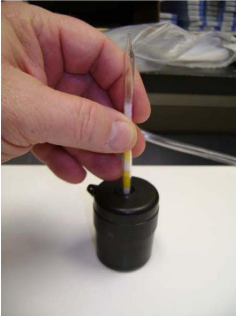
8) Insert the tube into the black rubber fitting on the low-flow adapter as shown, with the arrow pointing towards the tubing. The sorbent is close to one end of the tube, this is the end that should go towards the sampling pump. The tube shall be held or attached in an approximately vertical position with the inlet either up or down during sampling;
