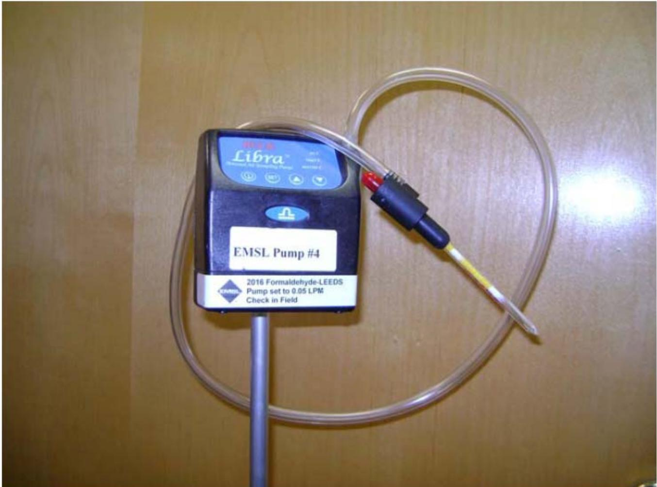
12) Periodically check to ensure that the pump is running. A pump that has failed and was left unattended during the sampling period will need to be discarded;
