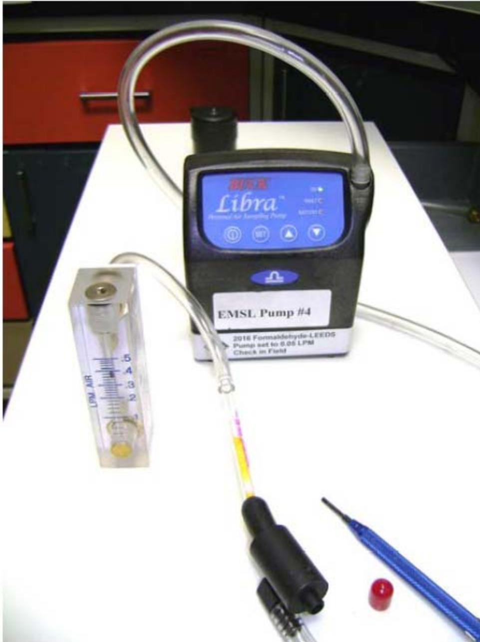
...and read the flowrate. It should be between 0.05 and 0.5 Liters per minute (lpm), the **OPTIMAL** flowrate is **0.3 lpm**. If it is not at 0.3 lpm, carefully use a small screwdriver to adjust the flow using the screw on the low-flow adapter **FIRST**;
