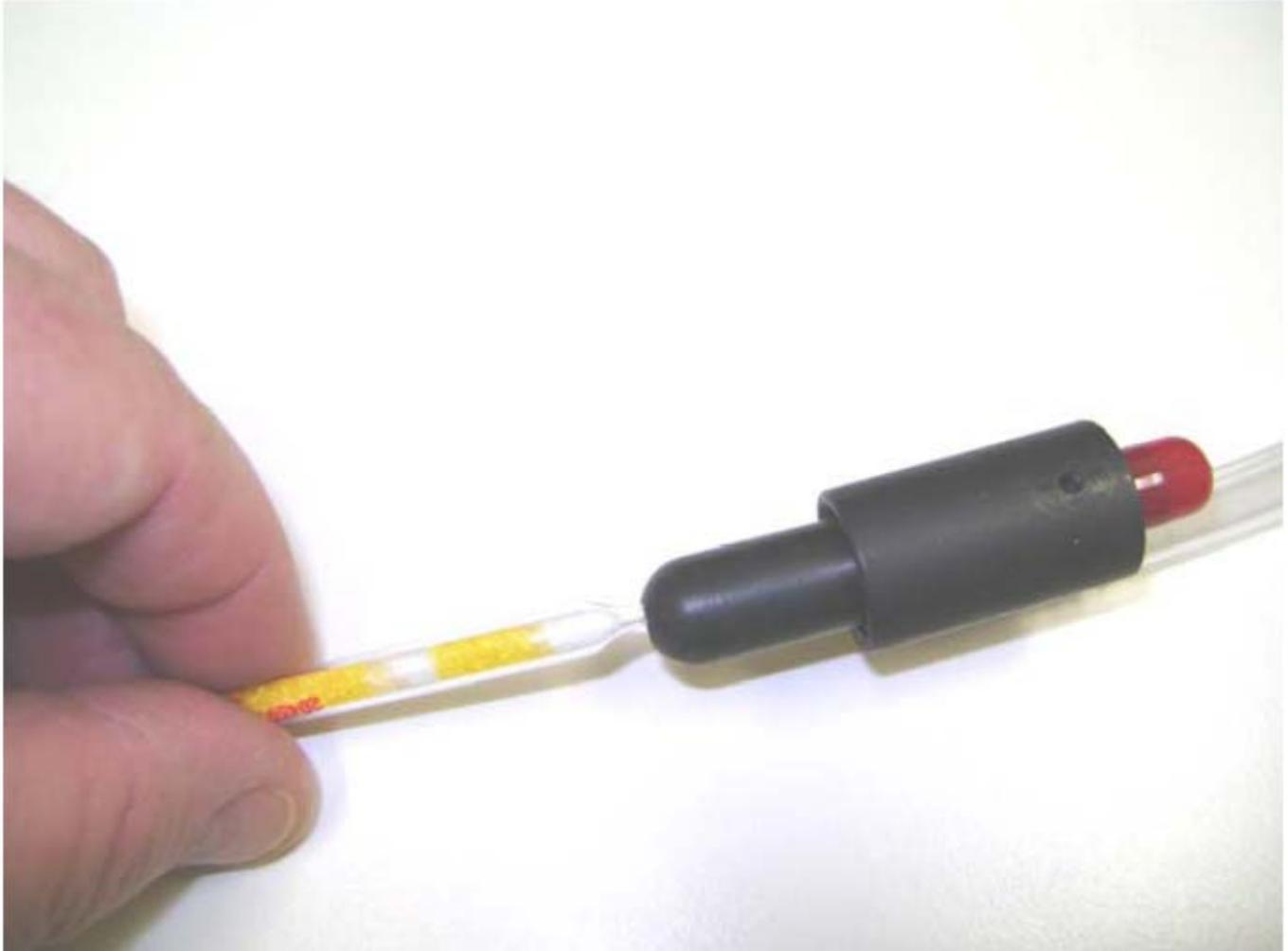
9) Turn the pump on (the LED light should turn on and you should hear the motor) – if it sounds like the motor is strained or frantic, you may have kinked the sample line or forgotten to break the ends off of the sorbent tube (see step # 7);
